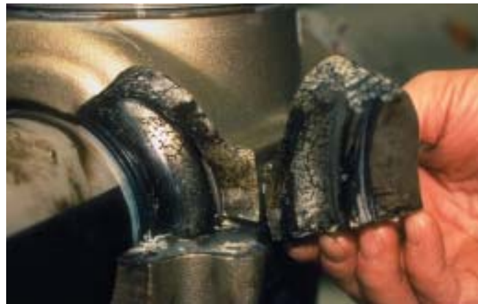
A cracked aluminum hub
