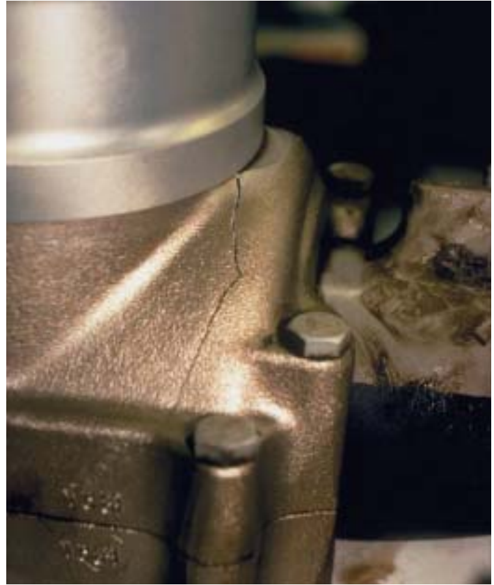
A cracked hub
