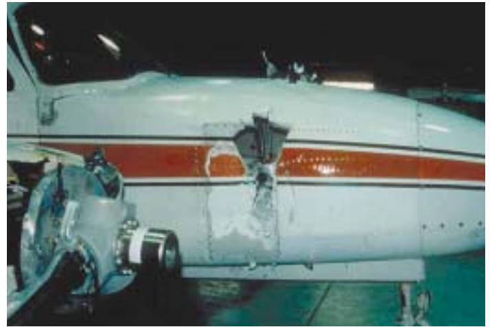
A catastrophic hub failure that allowed the blades to depart and puncture the nose.
