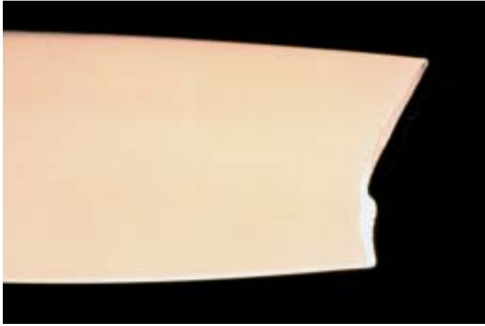
Missing blade tip
