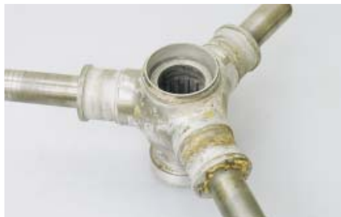
Corroded steel hub
